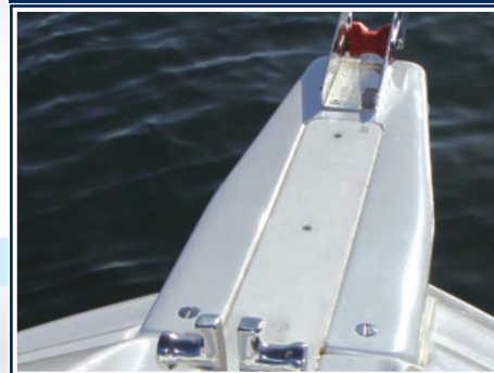
Heavy duty bow sprit includes teflon strip to protect against anchor chain damage
